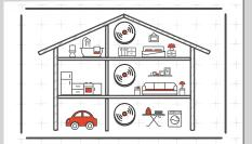
Install smoke alarms 10 feet from cooking appliances to minimize false alarms
