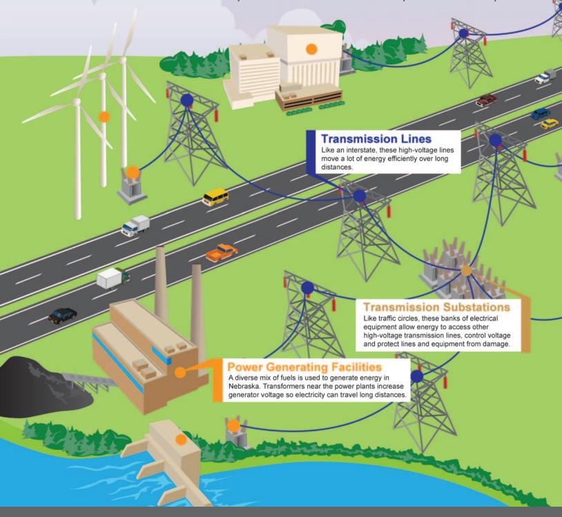
through a substation where the voltage is reduced, allowing the electricity to flow on to smaller distribution lines. These distribution lines carry electricity closer to its destination where once again the voltage is stepped down by a transformer to the 120 volts that you use in your home.
