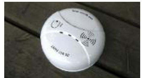
Installing a carbon monoxide detector near your natural gas or propane water heater is a critical safety measure.
