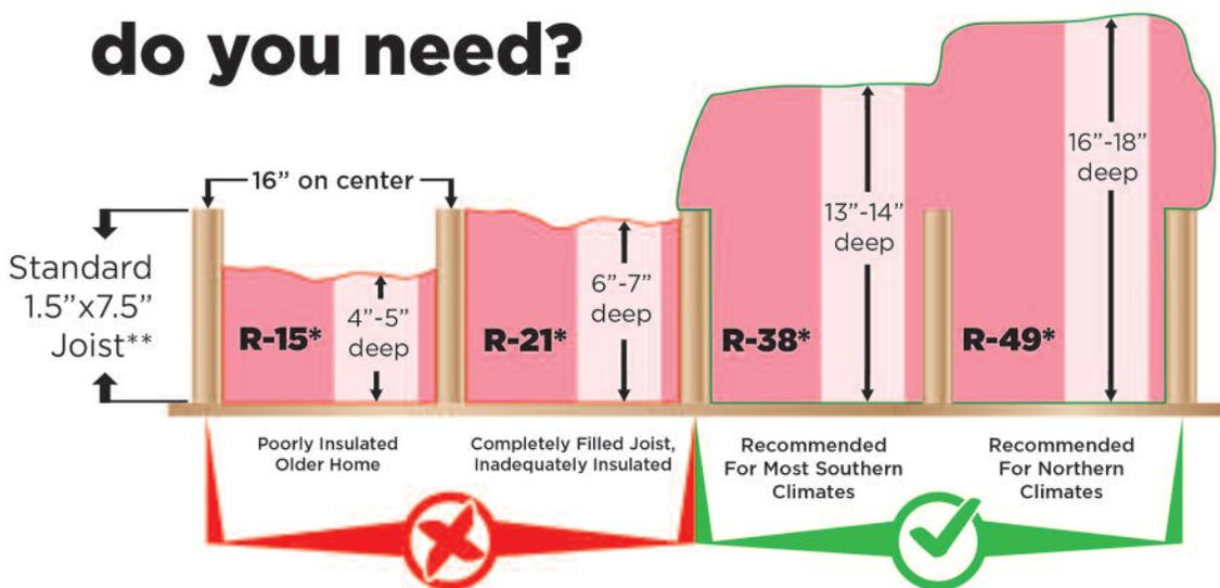
\* Recommended Dept. of Energy attic insulation levels for commonly used fiberglass, mineral wool, and cellulose insulation assuming about R-3 per inch.
